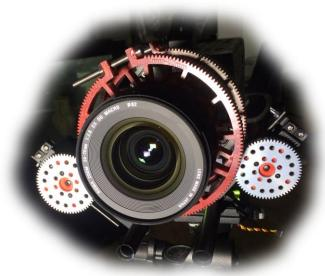
The system uses servos for lens control from a simple software application via Ethernet.
